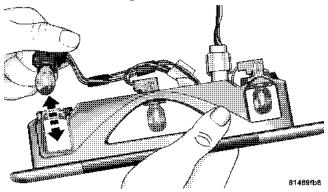
**Removing Socket From Housing**
